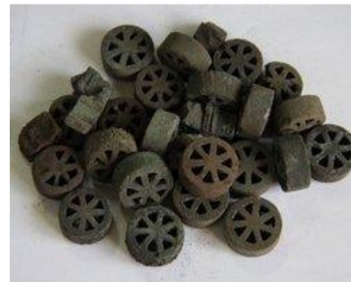
Katalizator reformingu benzyny Pt /SiO 2 Rh/SiO 2
